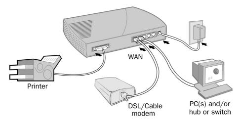
Figure 3: Installation Diagram
